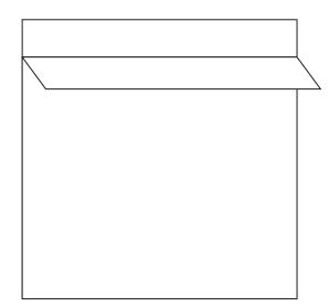
Carefully position sign on wall or window, placing exposed top adhesive area on to the surface.
